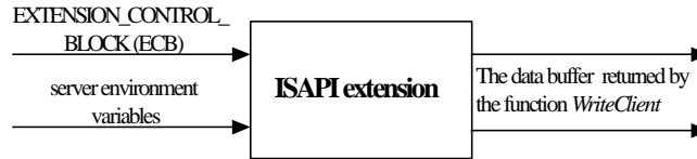
Figure 3. The scheme of ISAPI extension
